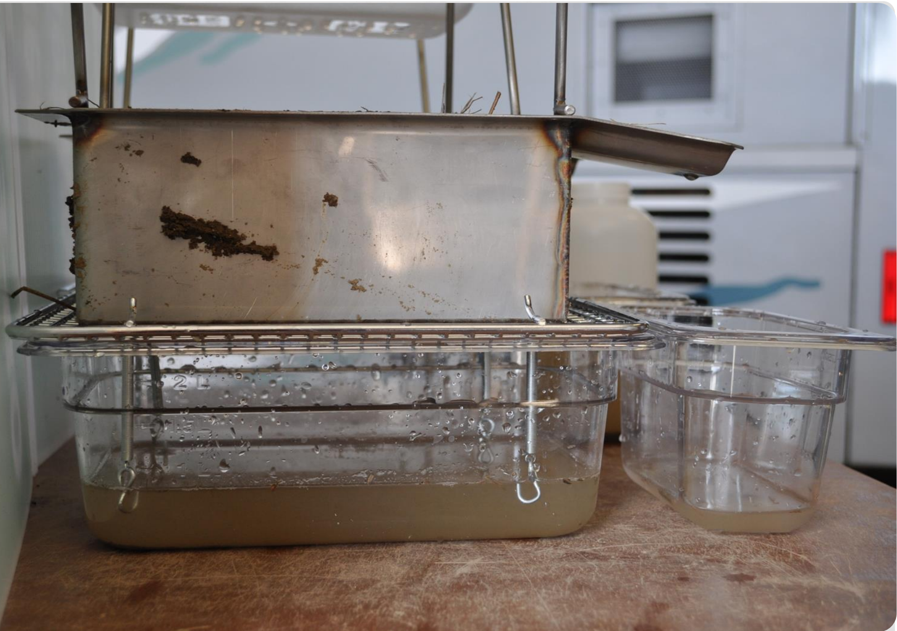
Gypsum Treated Soil: most water infiltrated, very little runoff
