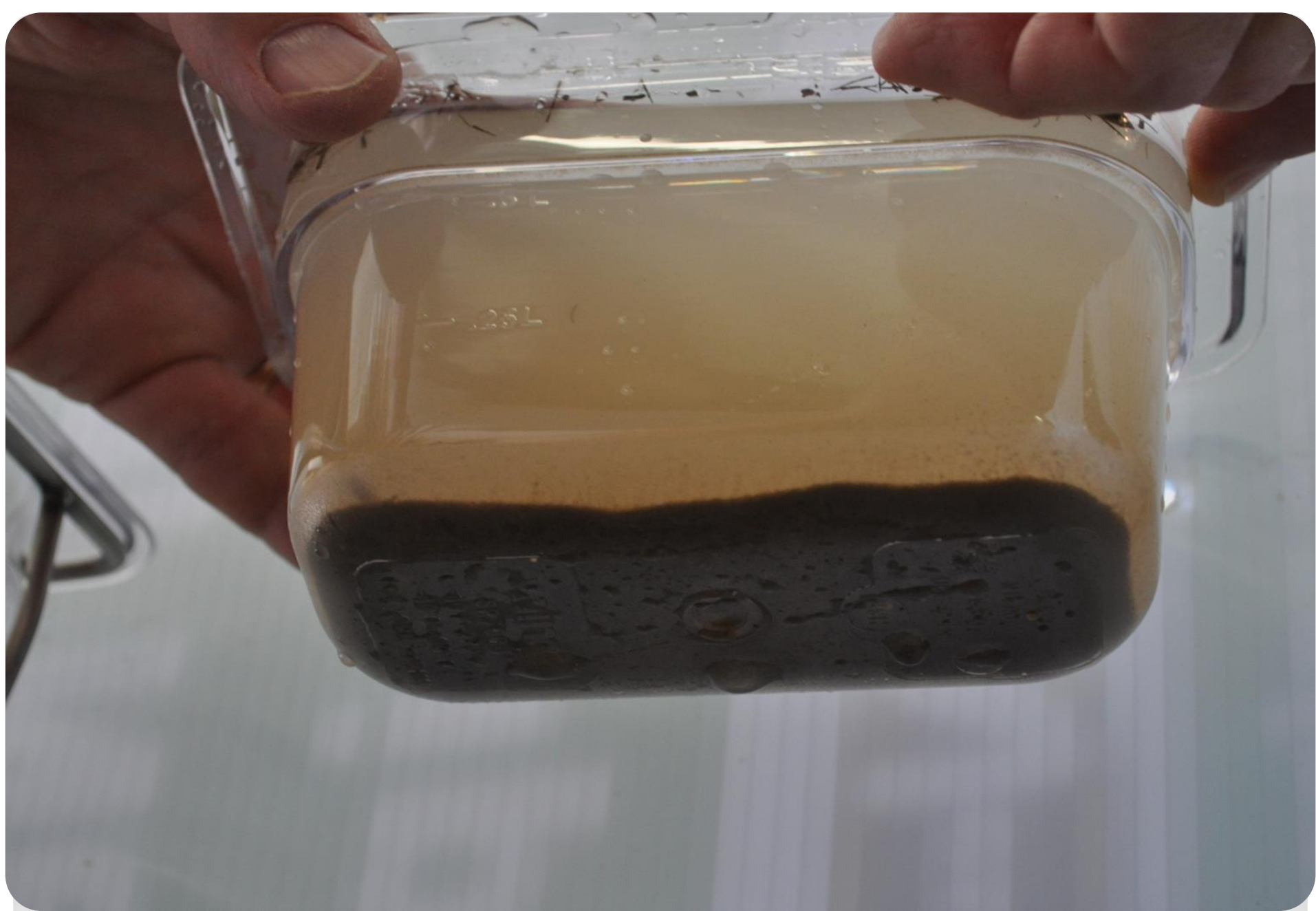
Control Soil: large amount of sediment in runoff
