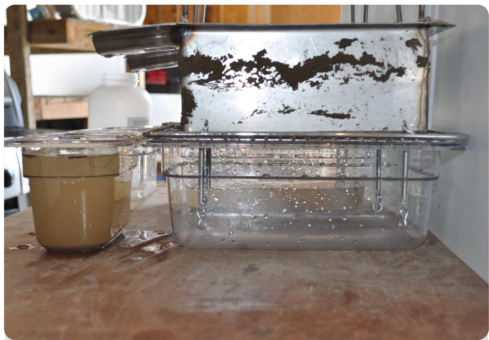
Control Soil: mostly runoff, very little infiltration
